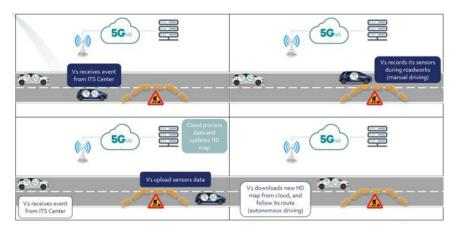
In this use case, the blue lead autonomous vehicle is driving on the motorway and receives a message from the ITS Centre notifying it of a road works event.
