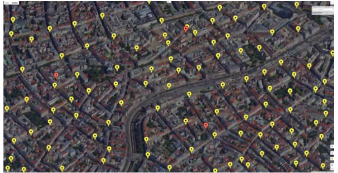
Fig. 1. Ultra-dense network deployment in Vienna city based on HetNet layout of [8]. Macro BSs and small BSs are denoted by red markers and by yellow markers, respectively.
