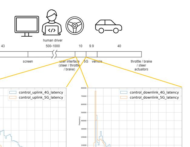
Communication delay only small part of entire pipeline (~10 – 17 [ms] of total ~220 [ms] (without human in the loop))
