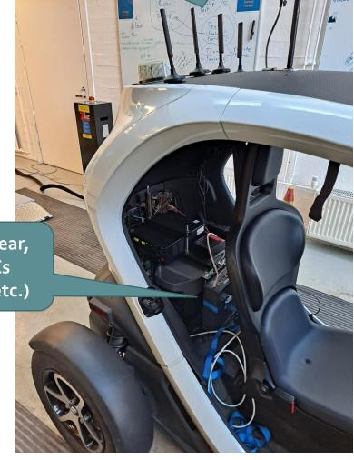
OBU deployed in rear, connected to PCs (vehicle, KPI tool etc.)
