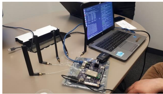
Figure 81: VEDECOM 5G OBU testing with Bouygues 5G network
