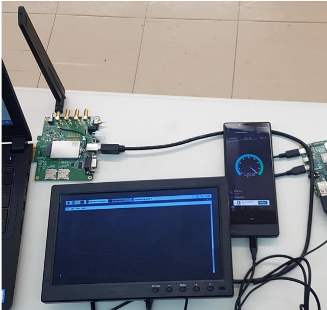
Figure 39: WINGS OBU & testing board under test in COMOSTE premises, Athens
