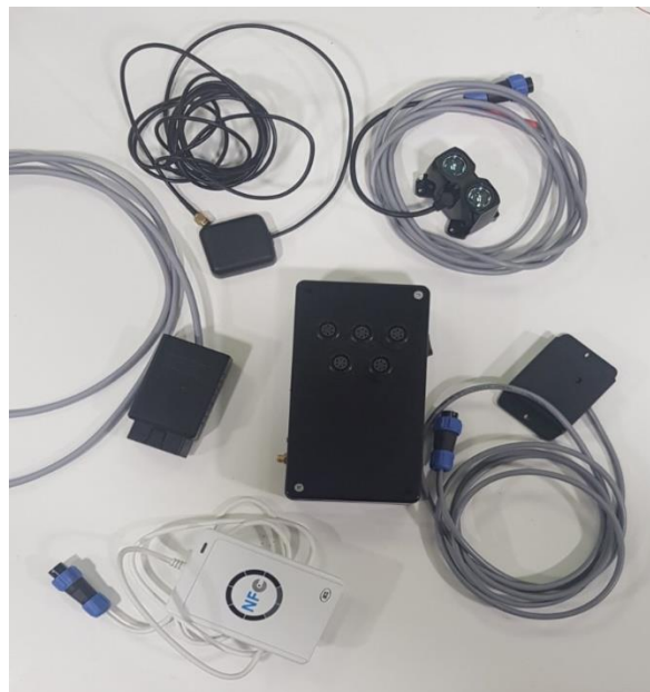
Figure 34: WINGS OBU (with integrated 5G chipset) & connected on-board sensors
