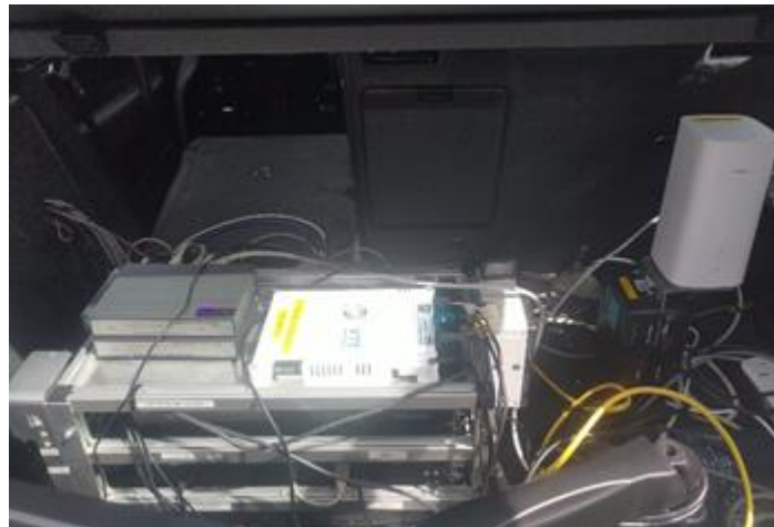
Figure 71: VTT OBU integrated in the trunk of the prototype vehicle Martti
