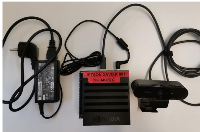
Figure 35: Jetson Xavier and Logitech USB camera used for the live streaming.
