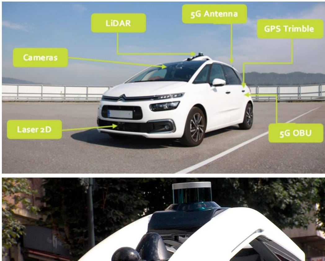
Figure 2: Overview of the Citroen C4 Picasso with all sensors
