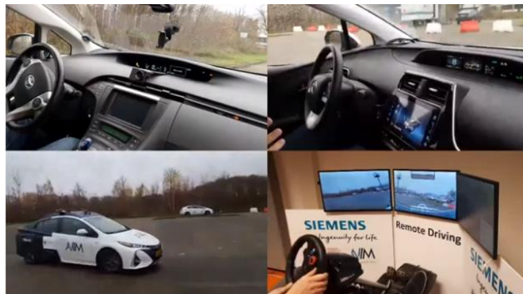
Figure 72: Screenshot of TU/e-AIIM and SISSBV vehicles remotely driven over KPN 5G SA network during PO review 3 December 2020
