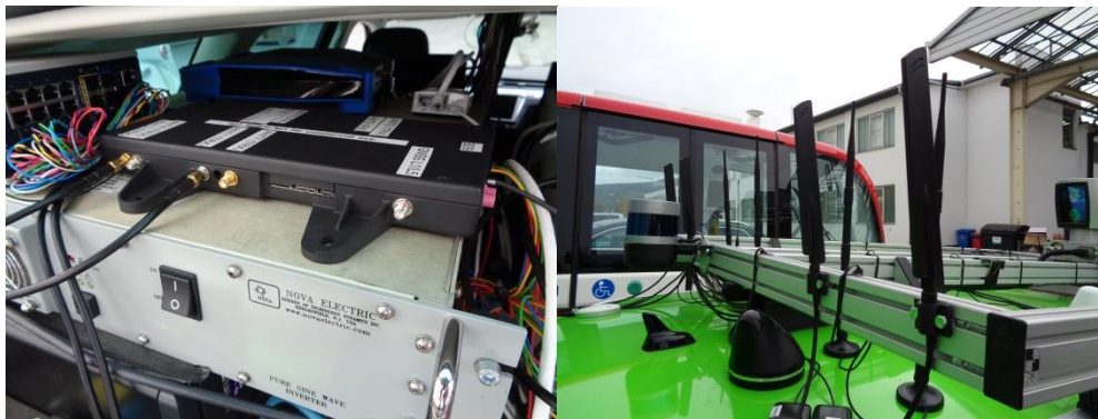
Figure 56: Integration of the OBU and antenna system on Valeo's VW Passat
