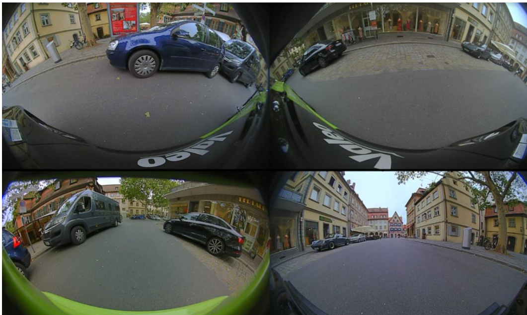
Figure 50: Raw images of fish-eye cameras. From top-left to bottom-right: right, left, rear, and front.
