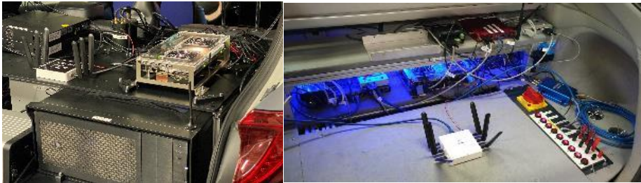
Figure 70: (left) TU/e-AIIM vehicle showing integrated OBU with 5G modem; (right) SISSBV vehicle showing integrated OBU with 5G modem.
