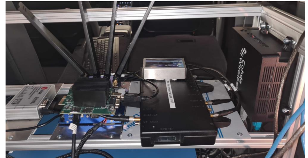
In-vehicle deployment of dual modem / dual SIM solution
